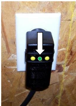
This Germination chamber is protected with a GFCI equipped cord. If the digital display does not come on when the cord is plugged in check that the reset button is set and the green light is on. Once the cord is plugged in the digital display on the thermostat will cycle through its startup routine. If the display does not come on check to make sure there is power at the plug and that the reset button has been pressed. Unplug the germination chamber for storage or to turn off the thermostat.
